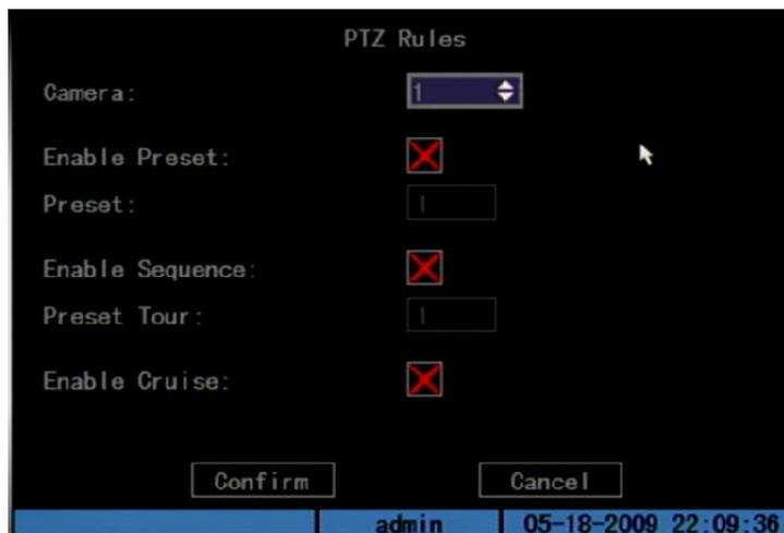
Select a camera, and then click one or more of following PTZ linkages: Preset, Preset tour, Enable Cruise (shadow tour). When an option is enabled, enter the number for the PTZ preset to be used. See “PTZ settings” on page 76 for more information on defining PTZ presets.
